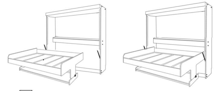
**INSERT TRUNION BOLT** Line up the trunion hole in the bed tray with the connecting 14 threaded hole at the upper end of the lever arm bracket mounted to the cabinet side panel. From behind the unit, slide the trunion sleeve and bolt through the hole in the lever arm bracket. Once both trunions are in place, use the 10mm allen wrench to firmly tighten the trunion bolts.
