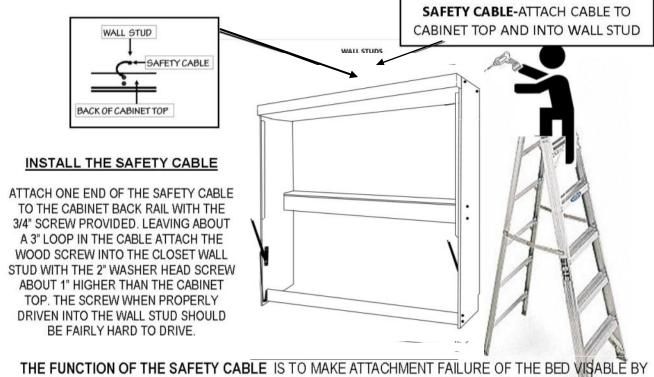
THE FUNCTION OF THE SAFETY CABLE IS TO MAKE ATTACHMENT FAILURE OF THE BED VISABLE BY ALLOWING THE BED TO COME AWAY FROM THE WALL 2 TO 3 INCHES. WHEN YOU SEE THIS CONDITION DO NOT OPEN THE BED! YOU MUST INVESTIGATE WHAT IS WRONG AND CORRECT IT!
