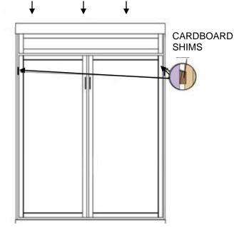
USING A STUD FINDER, LOCATE 3 WOOD WALL STUDS BEHIND THE BED AND MARK THEM WITH A VERTICAL LINE EXTENDING A FEW INCHES ABOVE AND BELOW THE CABINET TOP.WITH TWO PEOPLE TILT YOUR WALLBED INTO POSITION AGAINST THE WALL, MAKING SURE THAT ALL 3 STUD LINES ARE BETWEEN THE 2 SIDE PANELS. REACH OVER THE TOP OF THE UNIT AND DRIVE 6 -3 1/2" WOOD SCREWS THROUGH THE TOP ASSEMBLY BACK RAIL INTO THE WALL STUDS. NEXT, WITH THE BED OPEN, DRIVE THE ANCHOR SCREW THROUGH THE CABINET BASE INTO THE BASEBOARD.
