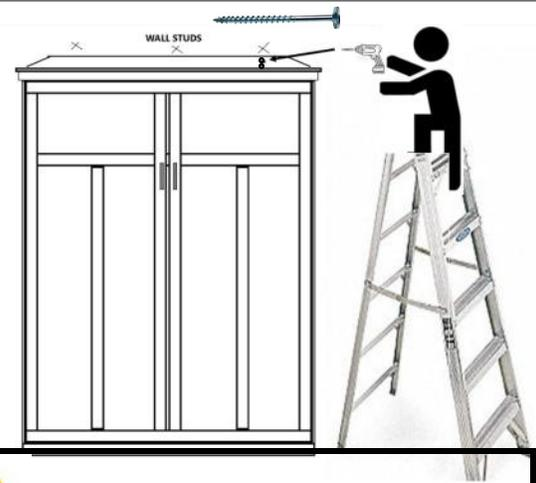
**!** If you are working with sheet metal studs, cinder block, brick, or concrete, you must provide three anchor points of 100 pounds strength each, before installing a Wallbed! **DO NOT ANCHOR TO SHEETROCK OR PANELLING!**
